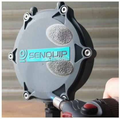
Flame-retardant materials reduce the risk of products catching fire and slow down combustion. UL 94 (Underwriters Laboratories test standard UL 94) is the most widely used flammability test for determining relative flammability for plastic materials. It measures the ability of plastic part to extinguish the flame after ignition.
